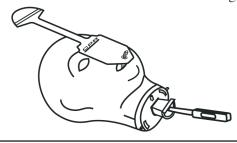
• Gently pull insertion tool until the bag extends out of the neck opening. Face shield portion should cover mouth.
